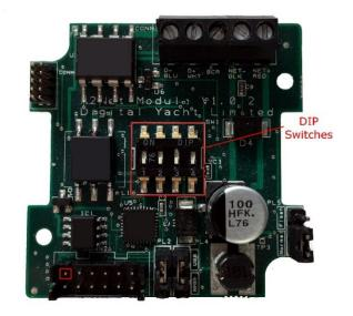
Once you have set the DIP switches, power cycle the veKonvert unit for the new Device Instance to be applied.
